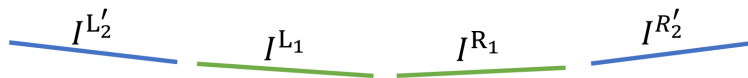
Figure 3: Diagram of generating images outside of the camera’s field of view. Green lines represent the true viewpoints of the two cameras, and the blue lines are the synthesized images. I^{L_2'} = G_1(I^{L_1}) and I^{R_2'} = G_2(I^{R_1})
